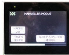
7" colour display + RFID & route module for programming options for RDIF-tags & routing Item no. OPTAGV0001
